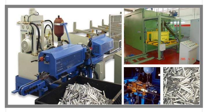
Fully Automatic Bar Shearing Machines with Bar Magazine, Automatic Feeder and Touch Panel for easy set up and to control the product length. All machines are easy and quick to set up and include a device for the separation of bar ends. We also design and manufacture automatic systems for 100% product length verification and automatic systems to fill and sort products in to containers.
